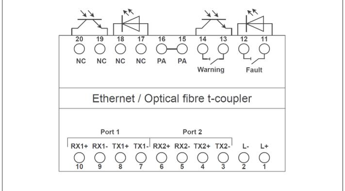
The use of 4-core Industrial Ethernet / Profinet cables is recommended, because there are no unused wires after connecting.
