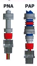
The PNA series cable glands are made of a metallic threaded body in which is put the EPDM seal (in red), pushed inside the body by means of a metallic nut and a metallic ring.
